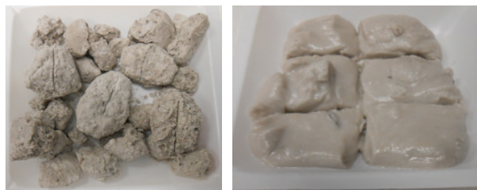
Evaporator scale without an inhibitor program.
