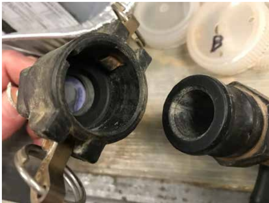
Figure 1: The inside of the cell where the deposit is placed at the bottom of the right side section
