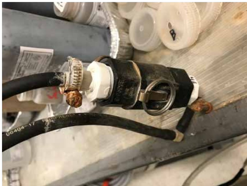
Figure 2: The recirculation-flow cell, which is placed vertically in the water bath, 60-80°C
